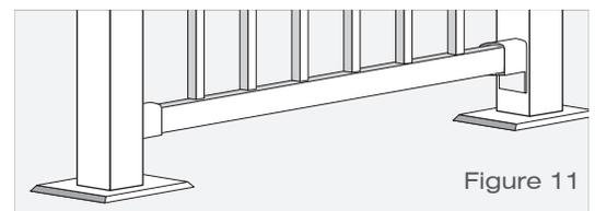
Top and Bottom Brackets are fastened to the Railing Spans with the White #10 x 3/4" Screws.
