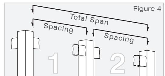
measurement needed for the next step. Fasten the Base Plates with the provided #14 x 3" Screws (with Clear Washers and White Snap Caps) to the deck for all the Posts in your installation.
