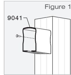
Top Brackets are fastened with #12 x 3/4" screws.
