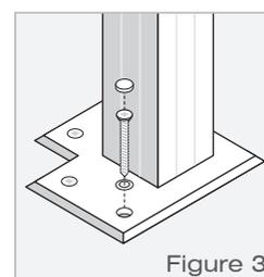
Base Plates are fastened with #14 x 3" screws. Cover with Caps.
