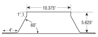
10" FLAT ROOF FLASHING
