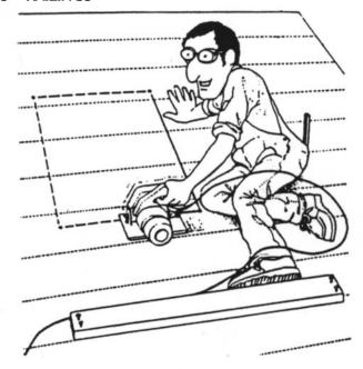
Cutting Through. Cut hole in roof to exact inside curb dimension listed for your skylite. Provision has been made for skylite contraction and expansion, but hole must be cut according to instructions to assume proper fit. Check local building codes before cutting any structural members.
