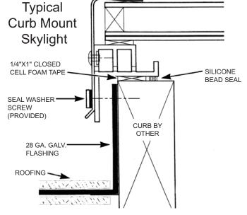
Flashing the curb. Install flashing as illustrated, up the curb to make a neat tight fit. Tack flashing to curb as necessary. One piece head & tail wrap around and seals corners of curb. Underlay shingles with flashing as roofing is built up along the sides of the curb. See steps 1-4 above.
