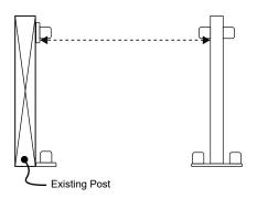
Measure from face of Base Plate mounted to Existing Post.
